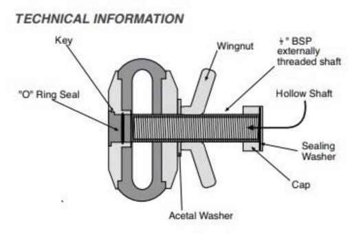
As can be seen from the sectioned view, the unique assembly of the central waterway into the base plate via a snap taper fit and "0" ring seal provides a positive water and air tight joint. The provision of a friction reducing acetal copolymer thrust washer inserted between the wing nut and top plate facilitates easy expansion and
